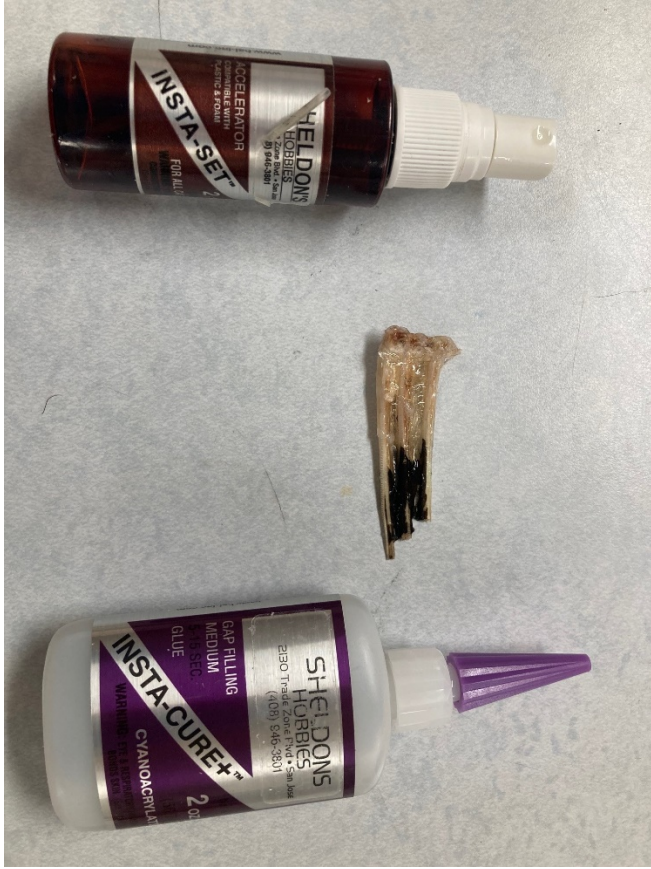
Appendix E5.—Insta-set and Insta-cure system for gluing fin rays.
