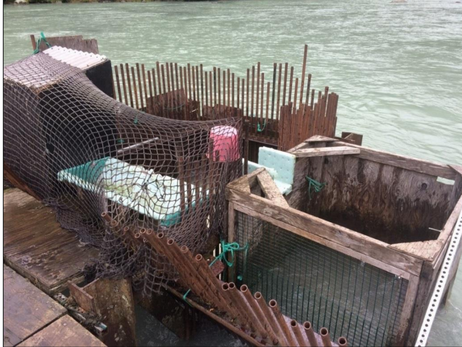
Figure 5.—Fish trap, recovery box, and fish sampling trough set-up at the Chilkoot River weir. (© 2019 ADF&G.)
