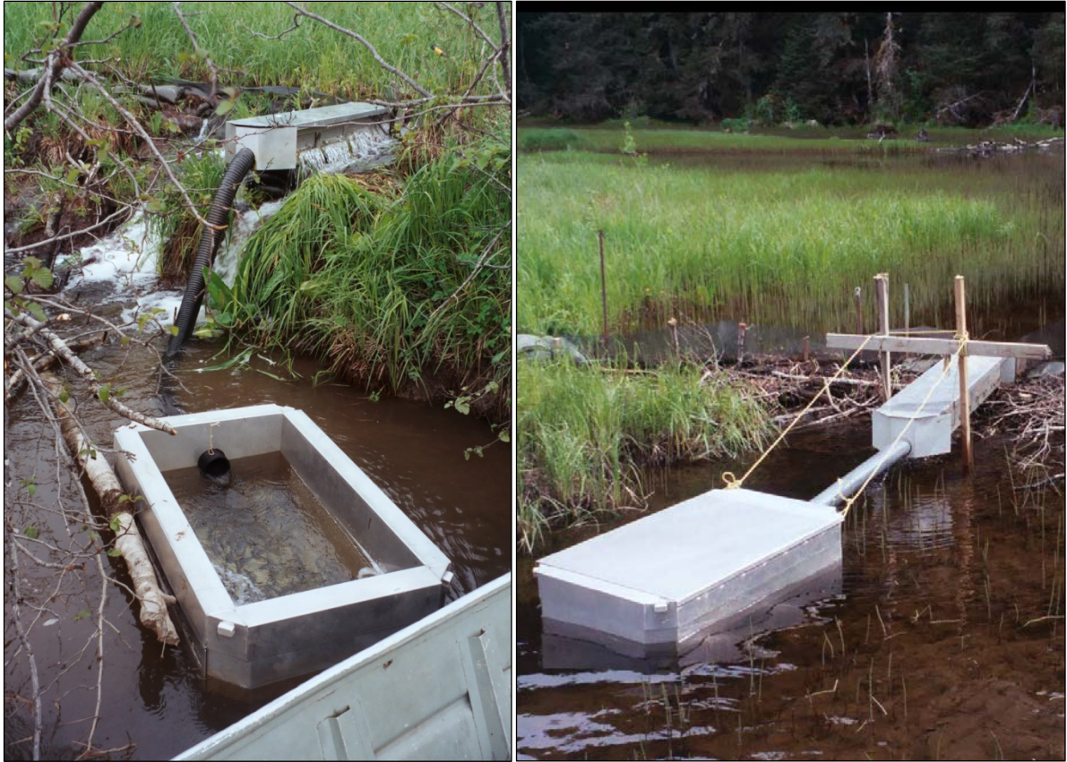
Figure 5.—Trough traps used to capture coho salmon smolts migrating over beaver dams at Shaul Pond and Det's Pond (©1997 ADF&G/photo by Leon Shaul).
