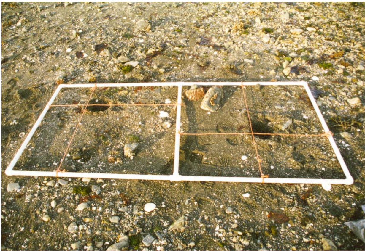
Figure 60. Fixture used to define the sample location in unseeded Control and seeded areas protected with plastic netting or seeded and left unprotected.
