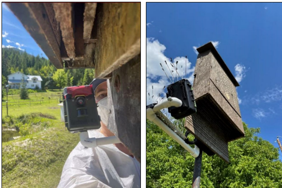
Figure 3. Monitoring occupancy at bat boxes using cameras. Infrared sensor on this game camera captures close-up imagery as bats emerge, triggered by motion. Susan Dulc (A) installs the camera off to the side of the landing platform just below the chamber openings (B). Blunt-tipped bird spikes are visible on gear to discourage perching birds that may harm bats. Photos contributed by S. Dulc.
